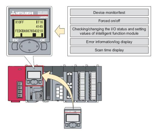
The display module is optional. The CPU comes with a blank plastic cover on the mounting location for the display module.
