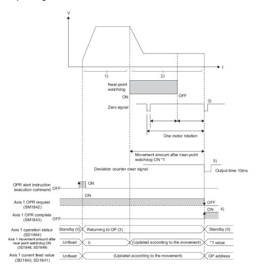
There is a special feature of OPR which can allow the controller to 'search' for the dog signal in the event that a limit switch is reached without finding the dog signal. This feature is called 'OPR Retry'. This function is always enabled when using the Near-Point Dog method, Count 1 method, or Count 2 method when limit switches for end of travel are enabled.
