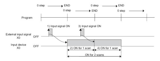
When a pulse input remains on for more than one scan, the program will only be provided with a one scan pulse. So the input in the program may turn off before the physical input turns off.
