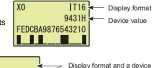
For word devices shown as 16-bit, the display is similar, showing all 16 bits within the word and a numeric value.
