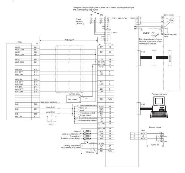
The pin numbers shown above for the LCPU are for axis 1. The pin numbers are different for axis 2. Axis 2 signals are found at the same numbers on the A set of pins in the connector.
