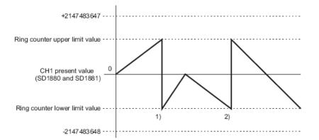
The **ICRNGWR1** and **ICRNGWR2** commands are used to set the upper and lower limits of the ring counter function. This command can only be used when the ring counter function is enabled on the normal mode counter.
