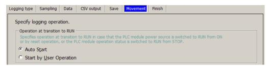
If Start by User Operation is selected, the software will have to be used to start the logging operation.
