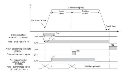
During the speed control portion of the movement, the current feed value is set to zero and not updated. Once the positioning portion of the control begins, the position will be updated.
