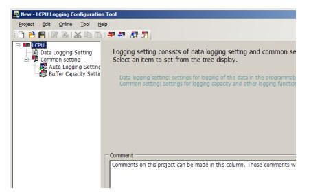
Click on Data Logging Setting in the left navigation window to display the list of configured data logging settings.
