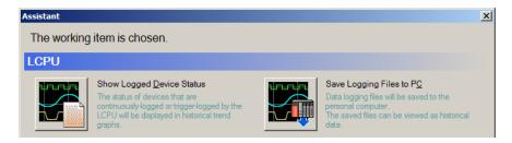
Select Show Logged Device Status and a window will open to verify transfer settings for communication with the PLC. Next is a screen showing the available logs in the CPU's memory card. This screen is identical to the one shown previously to view files on the memory card.
