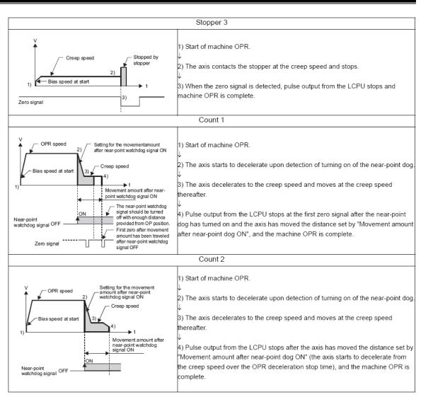
Machine OPR performs the actual movement to the home position and setting of the home position based on the method selected from the choices above.
