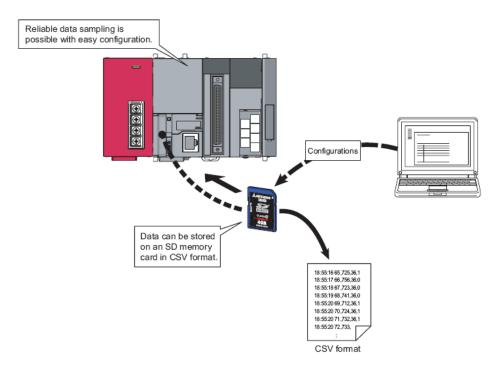
Some of the basic features of the built-in logging function are:
