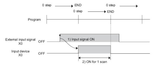
Inputs configured as pulse catch inputs should not be used as direct inputs (DX) in the program. They should also not be accessed with the input refreshing instructions, such as RFS, COM, CCOM, and MTR.
