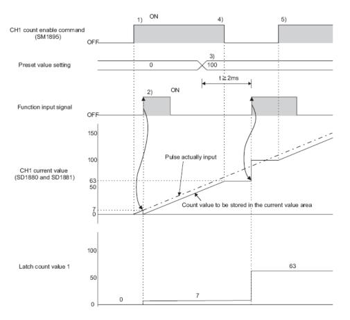
The latch count/preset function stores a value and resets the current value to the preset at the rising edge of the function input signal.
