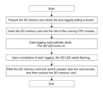
The conditions to indicate completion of auto logging can be set to either data logging stop or timer mode. When data logging stop is selected, this can be triggered by the completion of the specified number of samples in a trigger logging, the completion of the number of saved files in continuous logging, or the data logging being stopped from the configuration tool. In timer mode, samples will be stored for a specified time period and then completed.
