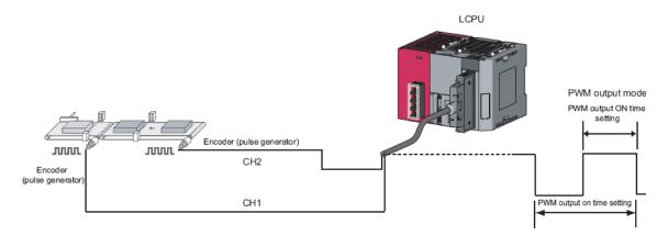
The current pulse count for a high speed pulse input is stored in a 32-bit location in the CPU. There are dedicated commands which are used to operate on this data without the limitations of the PLC scan time.
