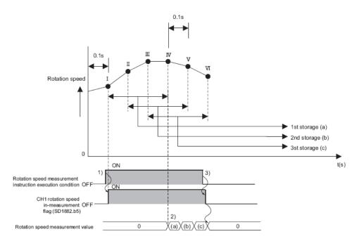
The commands **ICRCNT1** and **ICRCNT2** are used to read a rotation speed value. These commands are constantly driven while the rotation speed is to be read. This command is only available in the rotation speed measurement mode.
