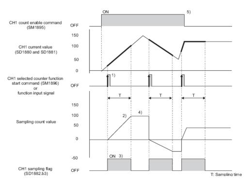
Sampling counter function is used to read pulses during a specified window of time.
