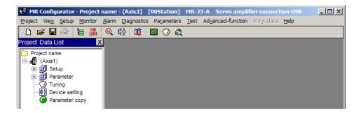
Across the top of the screen are drop-down menus and toolbar buttons allowing access to the various options of the software. On the left hand side is the project data list window, which is where the configuration data for the axis is displayed in a tree structure.
