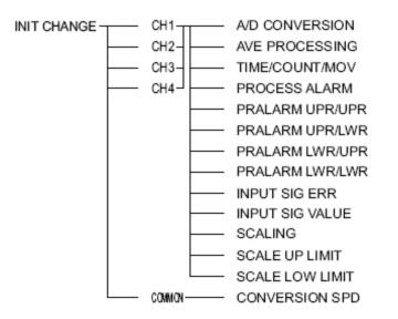
The menu tree below is for the LD62 or LD62D high speed counter input modules.
