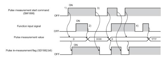
The commands **ICPLSRD1** and **ICPLSRD2** are used to read a measured pulse value. This command is only available in the pulse measurement mode. This command can be pulsed.
