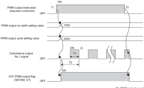
T1: PWM output on width setting value T2: PWM output cycle setting value
