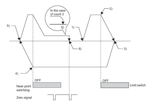
The commands **IPOPR1, IPOPR1P, IPOPR2**, and **IPOPR2P** are used to perform the homing of the axis. The commands ending in P are the pulsed versions of the commands not ending in P.
