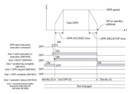
An error will be generated if a Fast OPR is attempted without the Machine OPR being performed.
