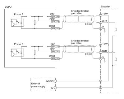
The example below shows the wiring required to connect a differential line driver encoder to the L Series CPU.
