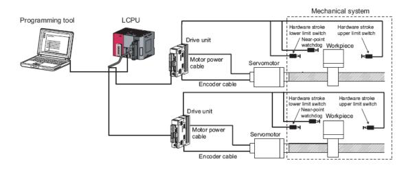
The L Series CPU offer 2 channels of high speed pulse output in the standard CPU. These 2 channels offer some basic functions, as shown in the list below.
