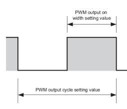
These values need to be set so that the output cycle value is greater than the on width value.
