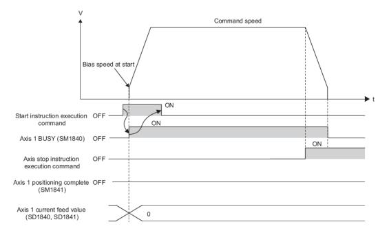
During the speed control portion of the movement, the current feed value is set to zero and not updated. Once started, the stop command must be issued to stop the axis.
